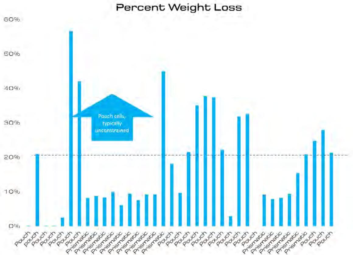
Figure 14 **Percent of mass loss as a function of cell form factor.**
