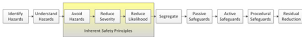
Figure 30. Hierarchy of Controls showing less effective controls such as active and procedural safeguards on the right of the figure. From Process Plants: A Handbook for Inherently Safer Design Second Edition ; Kletz, Trevor Amyotte, Paul; CRC Press 2010.
